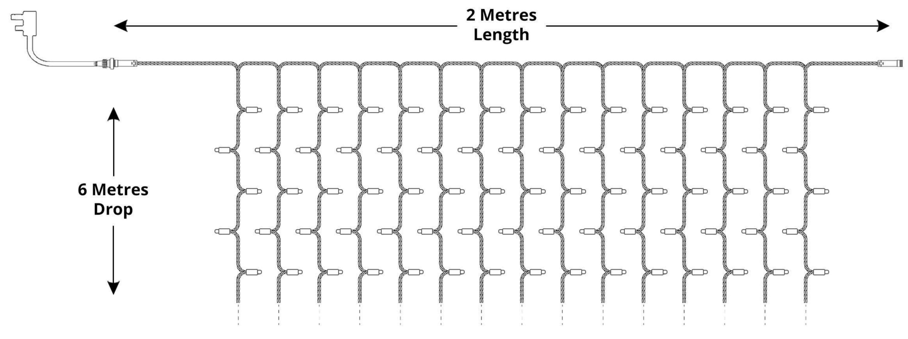
Connect up to 6 sets on one plug lead
