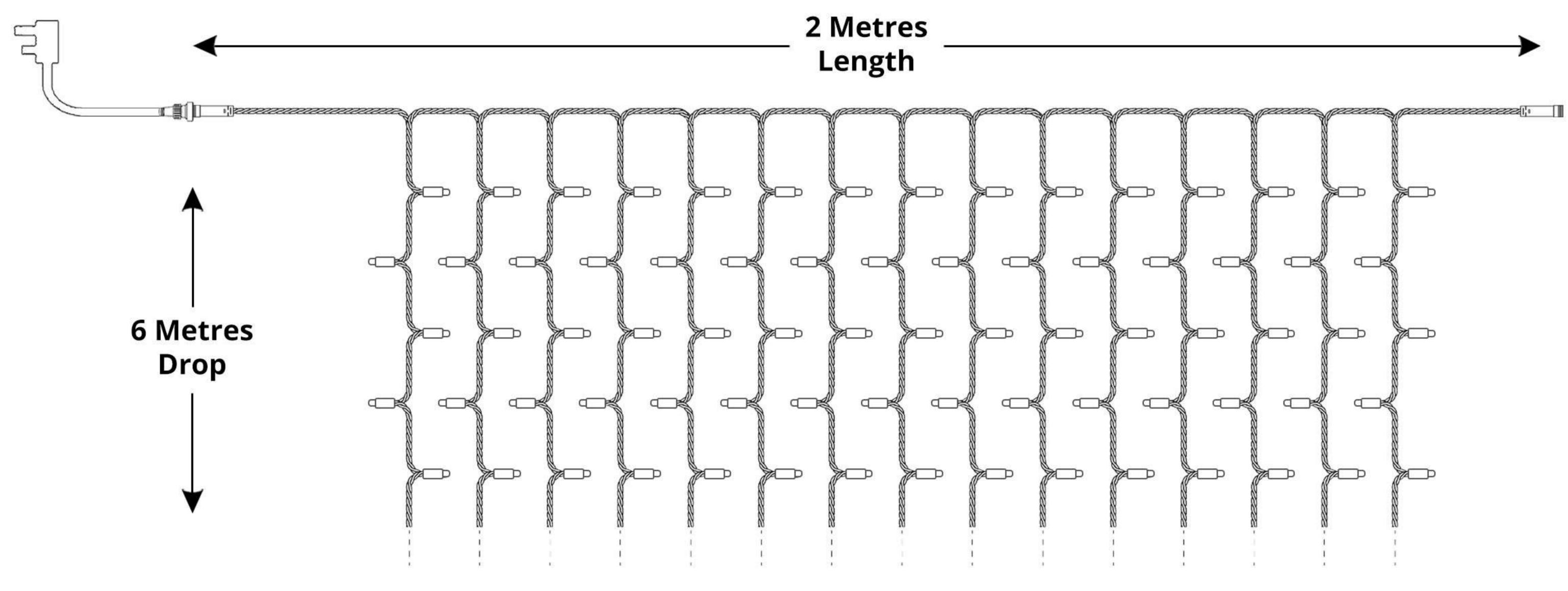
Connect up to 6 sets on one plug lead
