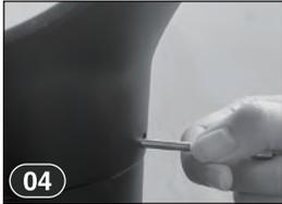
**04** Use the small screw driver to tighten the screw inside of light head to lock it tightly.
